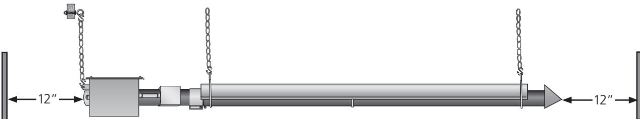
Figure 2.26 • Minimum End Clearance for Unvented Heater
